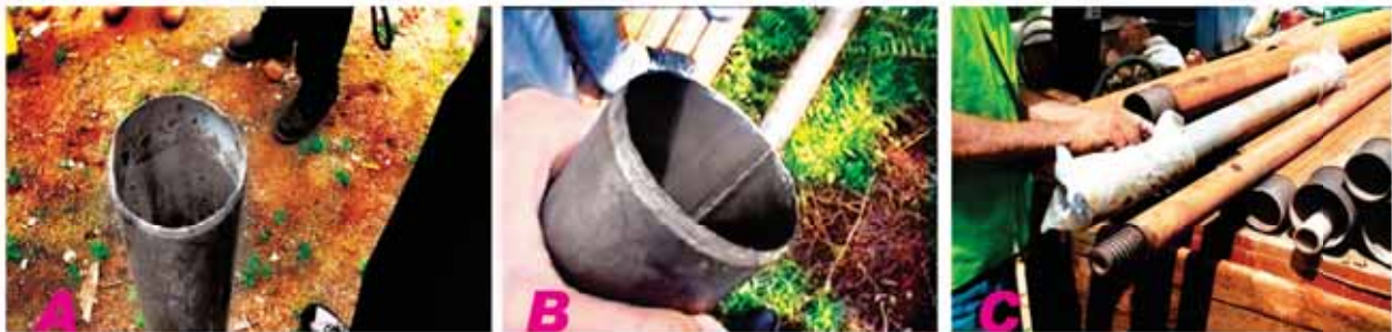
Figure 12c: Non-standard sampling tube with filed cutting edge and easily dented. (B) Sampling tube made out of exhaust pipe with obstructive seam on the inside. (C) Badly sealed and badly being transported undisturbed sample wrapped in loose plastic.
